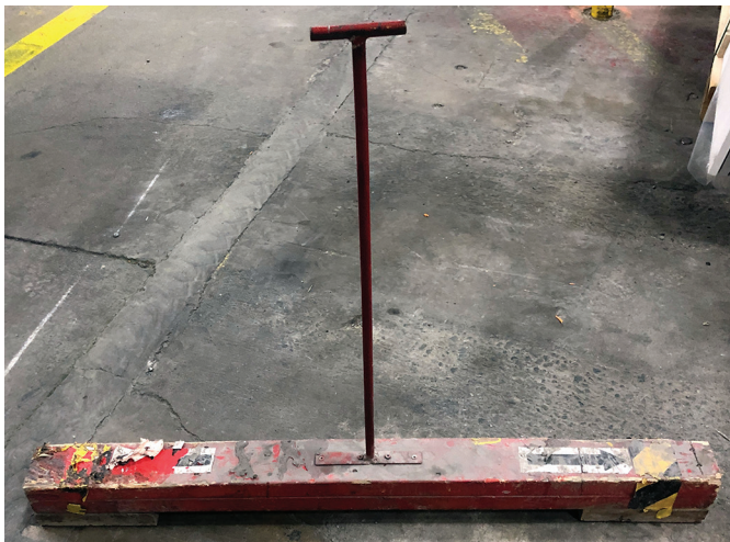
Figure C-2: Safety support for toe protection
