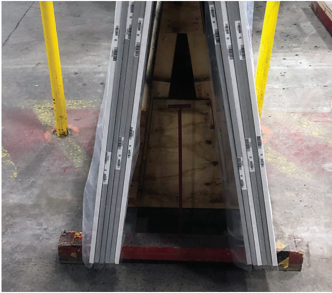
Figure C-1: Safety Devices (safety posts and safety support)
