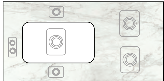
Figure F-2: Improper Suction Cup Support Placement
