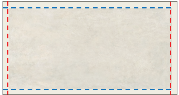
Figure C-1: Slab Trimming, Cut Long Sides (blue) First
