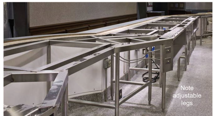
Figure J-4: Support Structure Example
