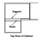
If a seam is made through or near the inside corner, seam reinforcement is suggested but not required when seaming with Corian<sup>®</sup> Joint Adhesive. Follow the guidelines for installing seam reinforcements.
