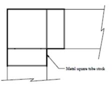
To test a design, apply a 100-pound (45-kg) weight to the inside corner as shown in Figure E-3. The maximum deflection allowed is  $^{1}/8''$  (3 mm).
