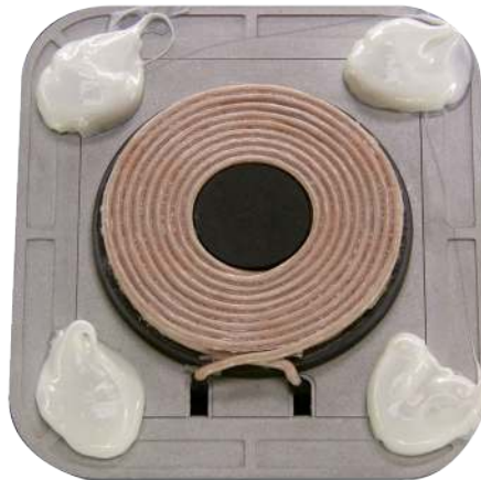
Figure D-2: 100% Silicone applied to transmitter
