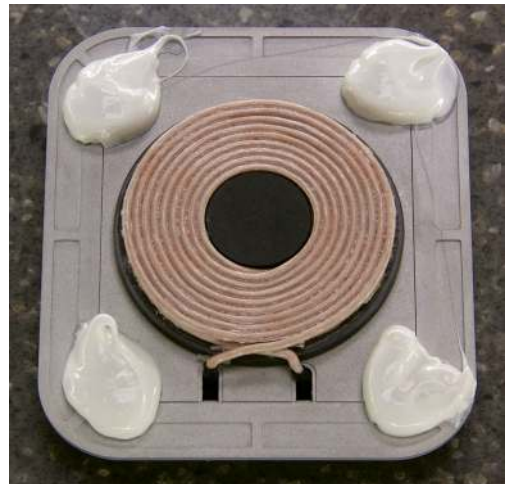
Figure D-2: 100% Silicone applied to transmitter
