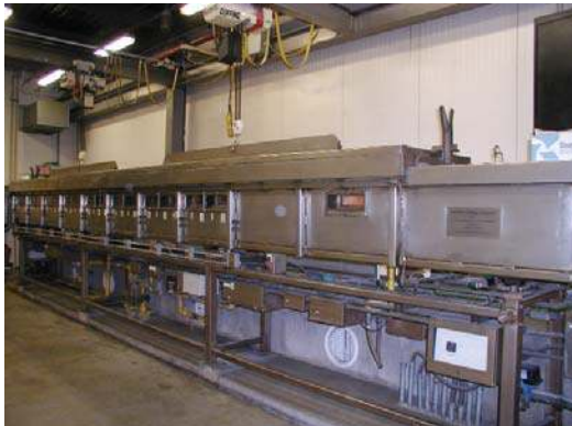
Figure II: Exterior view of the Steiner Tunnel apparatus: Underwriters Laboratories Inc., Northbrook Division, Northbrook, Illinois. Tunnel or chamber lid is in place. Operator uses viewing windows along the side of tunnel to quantify flame propagation.
