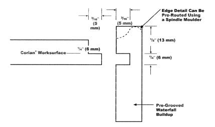
The no-drip detail can be premade using a shaper or alternatively can be done with a handheld router using a no-drip router bit as illustrated in Figure 12.13.B.
