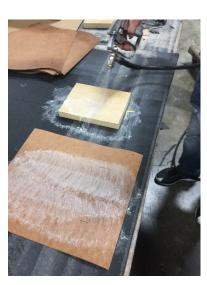
2 - Laminate the front surface and cut-out the outside corners as shown
