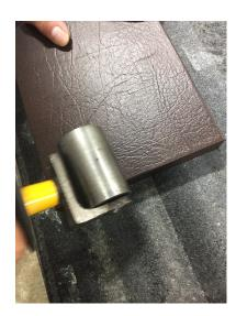
4- Apply a fill stick crayon of a matching color to fill the edge on the corner for a cleaner look.
