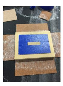
3 - Fold the leather on the panel, applying pressure with a hand roller on all surfaces. Cut out excess material.
