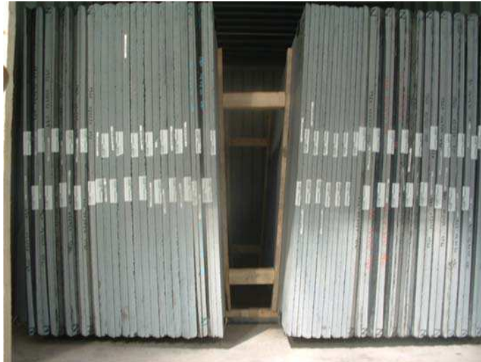
Typical Container Configuration with U-Frame
