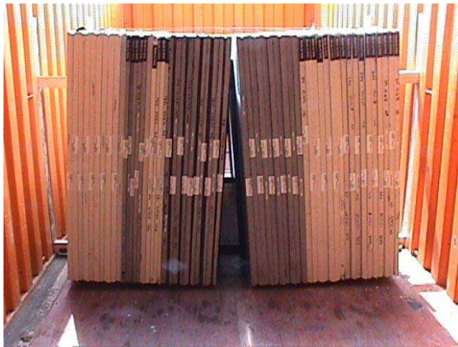
Typical Container Configuration with A-frame
